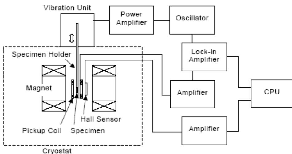
**Fig. 2. Scheme of a typical experimental setup for measuring the magnetic hysteresis curves of superconductors using VSM (Vibrating Sample Magnetometer) method**
