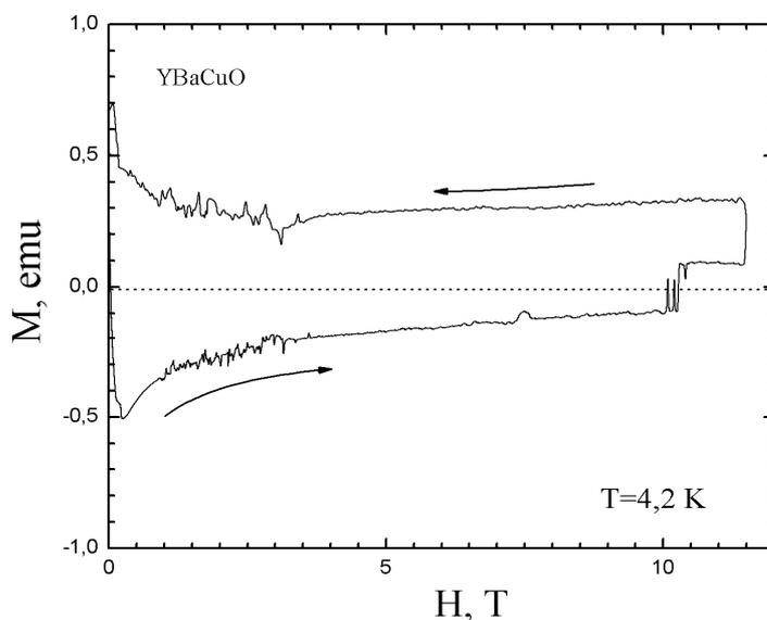
**Fig. 1. Hysteresis loop of the magnetization curve in high magnetic field, for sintered HTc superconductor  $\text{YBa}_2\text{Cu}_3\text{O}_{7-x}$  as a function of applied magnetic induction, with shown small flux jumps instabilities. Arrows indicate the direction of variation of applied magnetic field**
