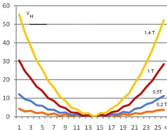
**Fig. 3. Profiles of the magnetic induction distribution, described by Hall sensor signal, along an axis of superconducting coil with HTc shield, for various maximal value  $B_m$ , given at each curve. X is number of the measured point along an axis of the coil,  $V_H$  is Hall probe signal, while all curves are pinned at their maximal values**
