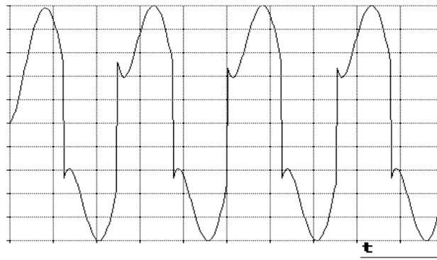
Fig. 4 The waveform of the load current
