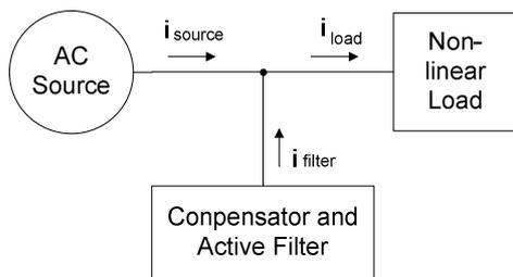
**Fig. 1. Basic scheme of parallel compensation and filtering**
