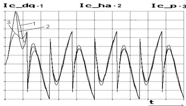
Fig. 5 Reference active filter currents computed by all three methods:
