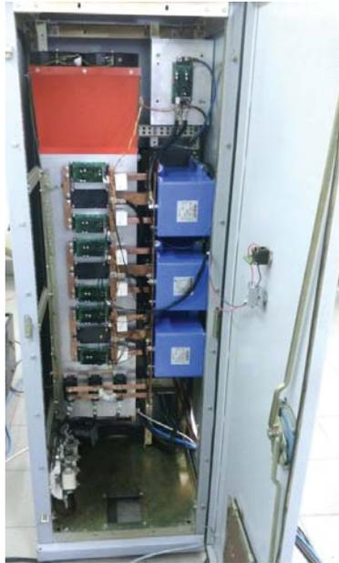
**Fig. 7. View of the laboratory three-phase three-level 55 kVA inverter**
