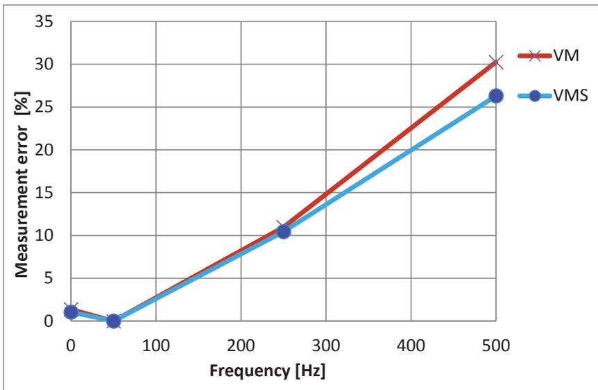
Fig. 6. Comparison of measurement error of the VMS sensor with a commercial sensor (VM)
