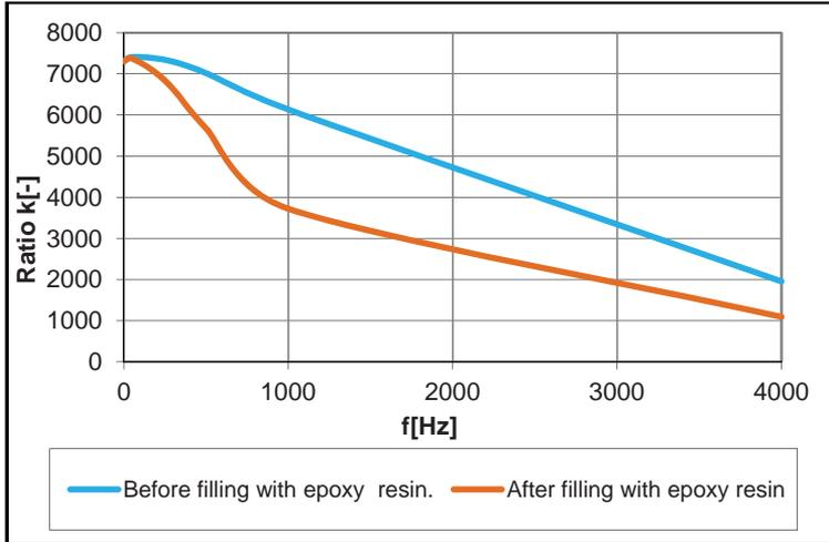
Fig. 3. Ratio of the voltage divider k in the frequency domain
