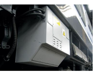
Rail static inverter type PT 3000/40 is a device for the conversion of electrical energy in a rail vehicle.
