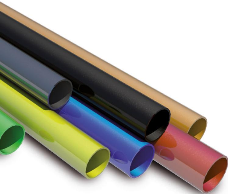
Glass-epoxy pipes are made by winding on metal cores saturated with an epoxy composition of glass fiber. The structure of the pipe is programmed. The direction in which the fibers are arranged in the layers depends on the type of load carried by the pipe, most often it is bending or torsion.
